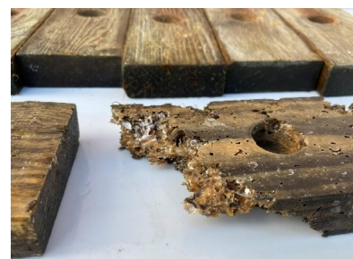
Shipworm damage in experimental wood
